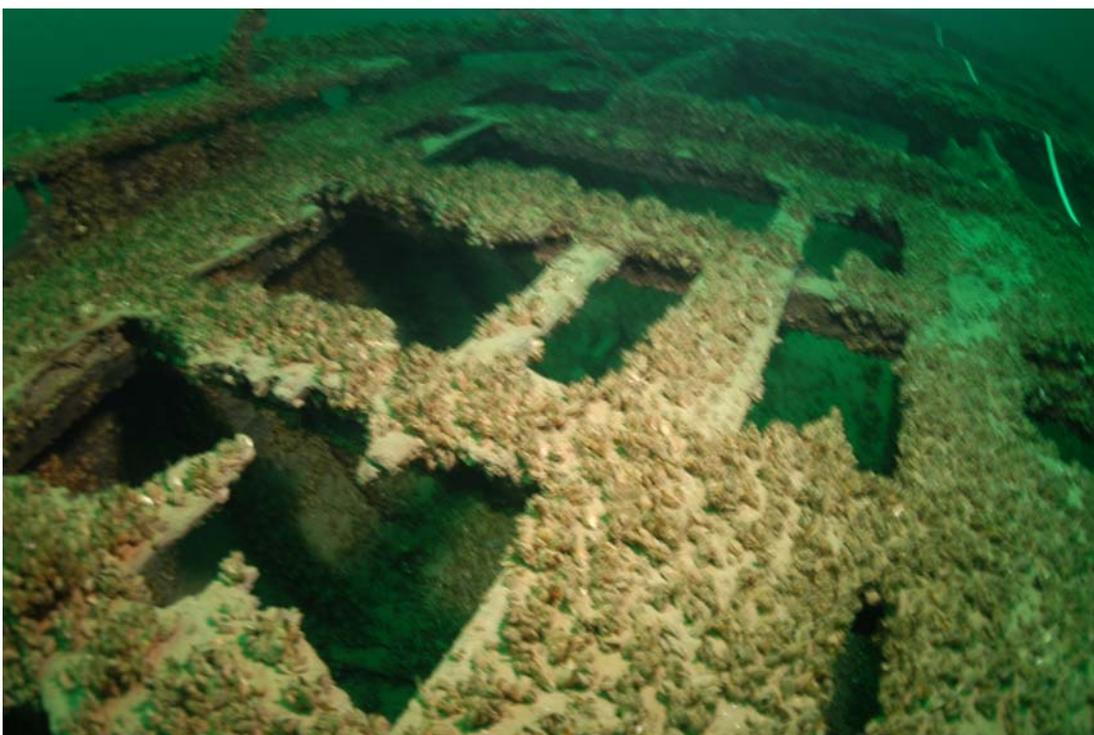
Figure 35. Deck beams and planks.
