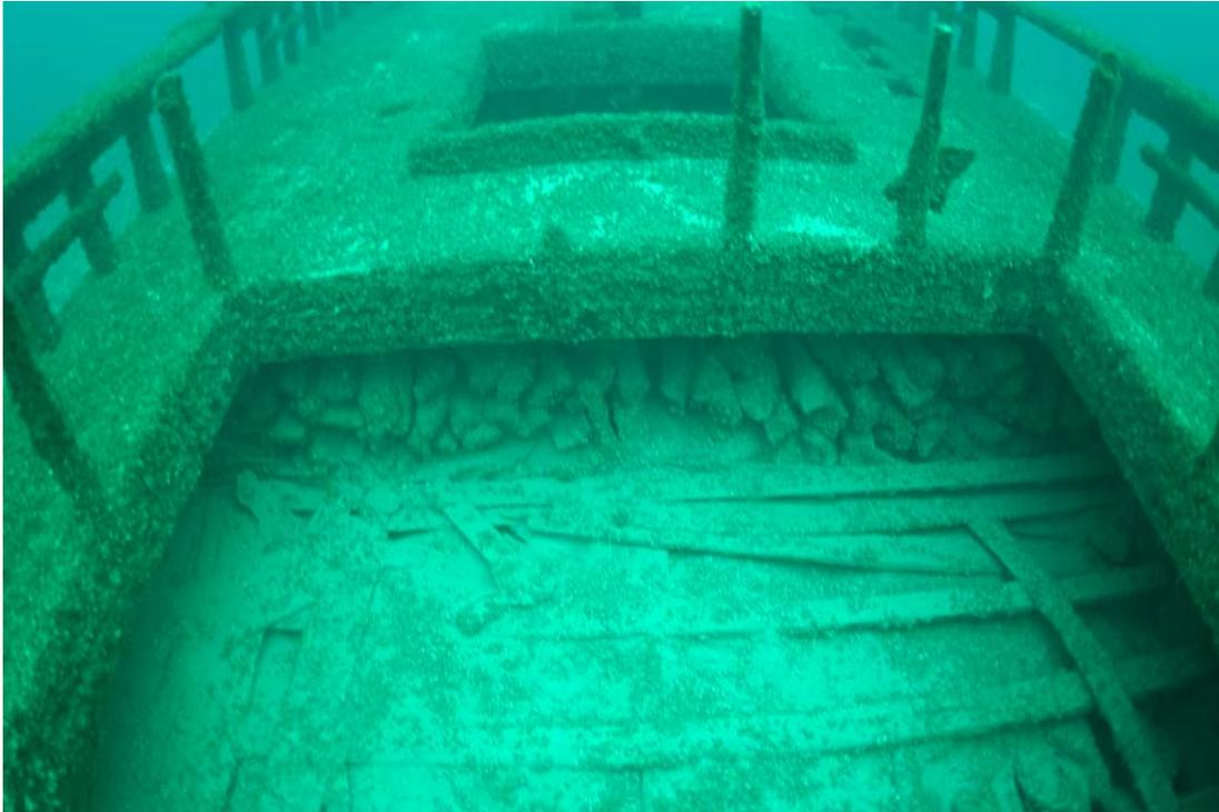
Figure 47. The cabin opening, looking forward. Frames for the cabin bulkheads are extant, and the wood cargo is visible, neatly stacked in the hold.
