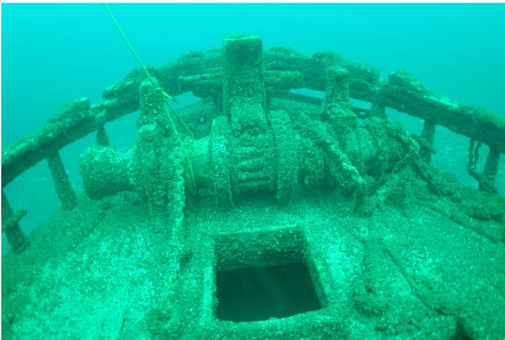
Figure 44. The windlass viewed from astern, with forecastle scuttle and deck pipes visible.
