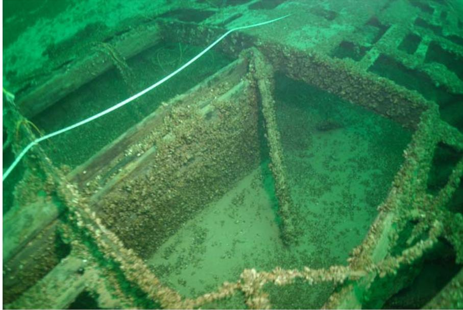
Figure 37. Centerboard and trunk visible through the cargo hatch.
