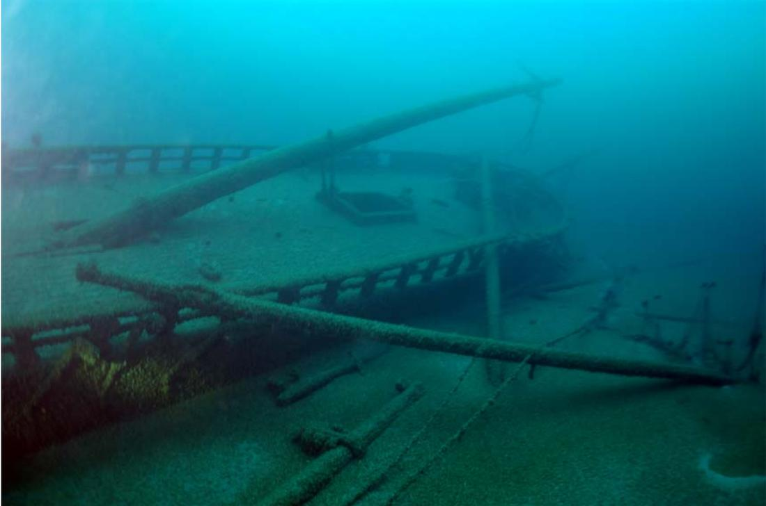
Figure 19. Many of the vessel's spars lie off the starboard side. The fore yard lies across the windlass, and a boom lies across the starboard rail. A topmast lies underneath the boom, with a gaff lying nearer the hull. A smaller yard is visible lying off the starboard bow. Most of the spars are tangled in fish net.
