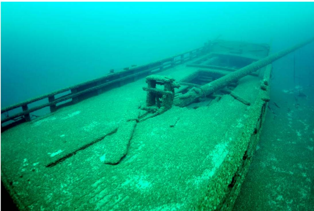
Figure 26. Centerboard winch, looking aft. The missing deck plank over the centerboard trunk is visible, as is the loose plank with chain attached.
