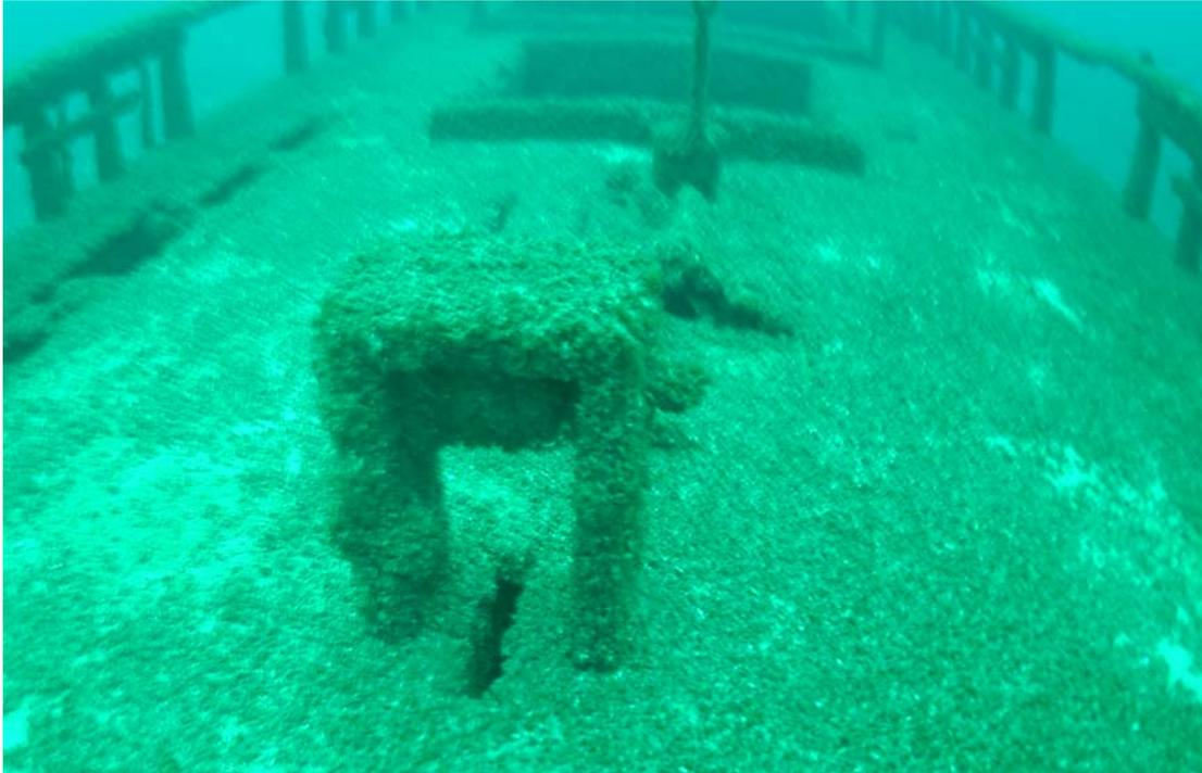
Figure 46. Centerboard winch and chain slot through deck, looking aft. The aft bilge pump is visible forward of the cargo hatch, as are the aft bulwark gaps on either side of the cargo hatch.
