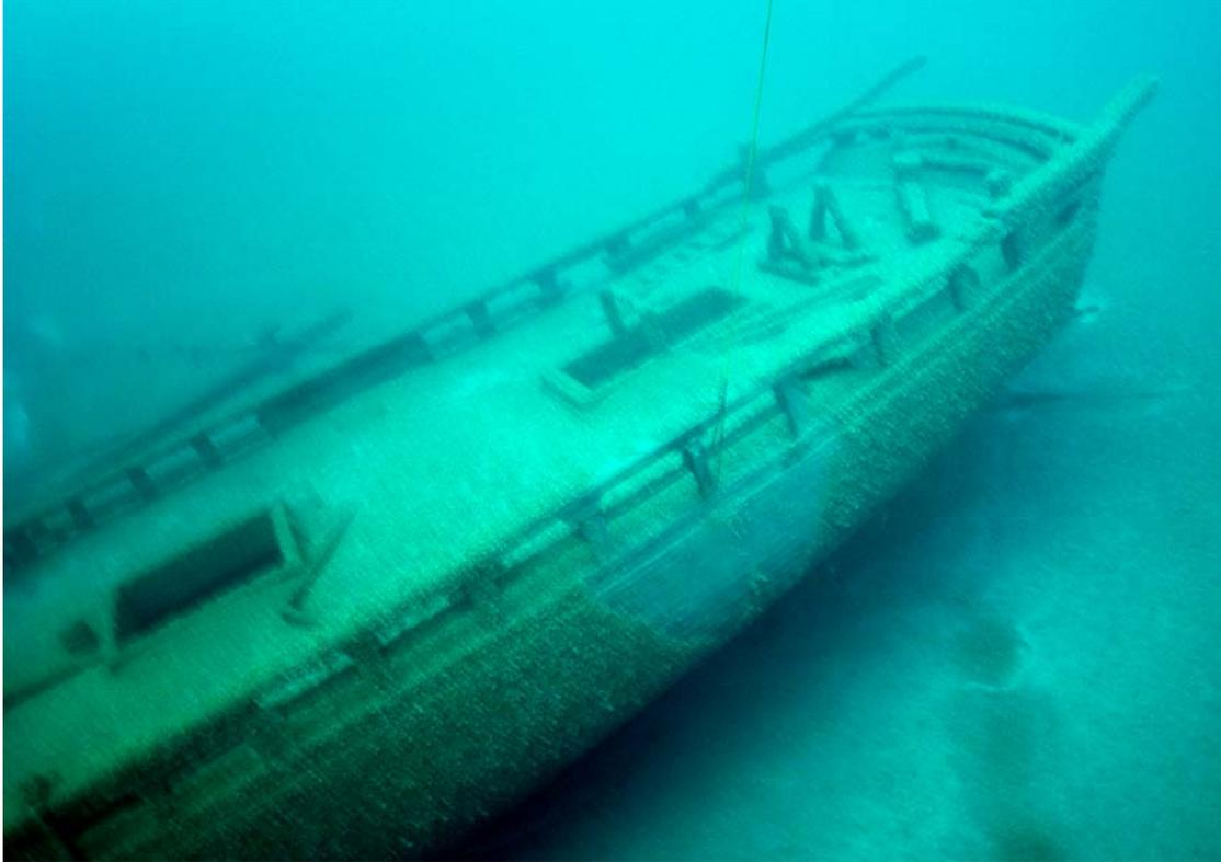
Figure 15. Stern deck arrangement with below-deck cabin. Note missing wheel.
